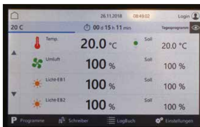
Control unit of an environmental chamber
