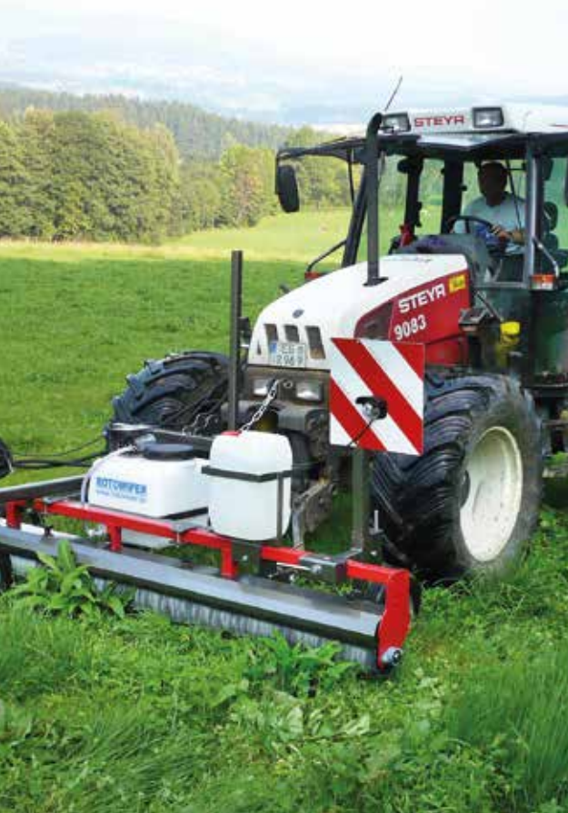
Controlling sorrel with a Rotowiper® weed wiper
