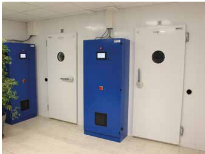
Two climate chambers offer plenty of space for germination tests with precisely maintained parameters
